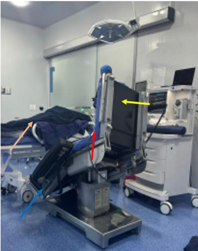
Figure 2: Surgical table with distal end elevation. View of the autonomous surgical table from a different angle, showing its malfunction position in the foreground.
