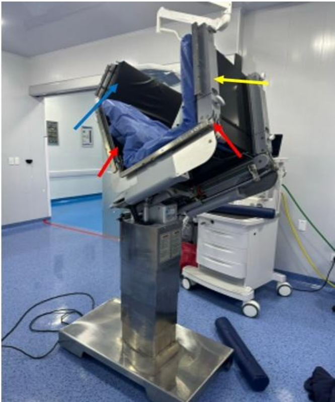
Figure 3: Surgical table in continuous movement, acquiring an elevated position. Red arrow: Show the direction of the unexpected table tilt. Yellow arrow: Point to the head section of the table. Blue arrow: Point to the foot section.
